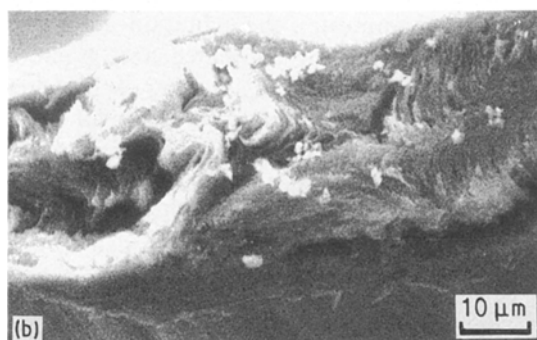
Figure 2 Comparison of the fracture surface morphologies of (a) a Pitch-55 fibre and, (b) the ribbon.
