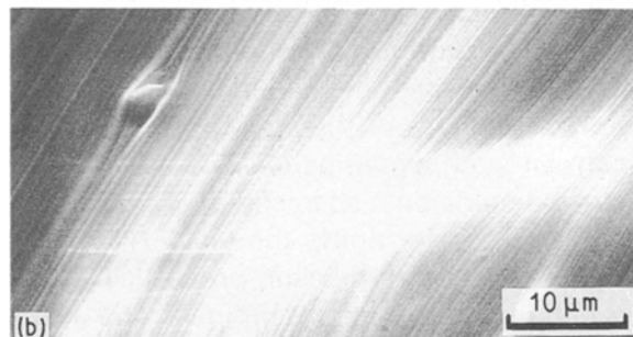
Figure 1 (a) Low magnification micrograph of the carbon ribbon showing structure inhomogeneities, (b) high magnification view of a typical inhomogeneity.
